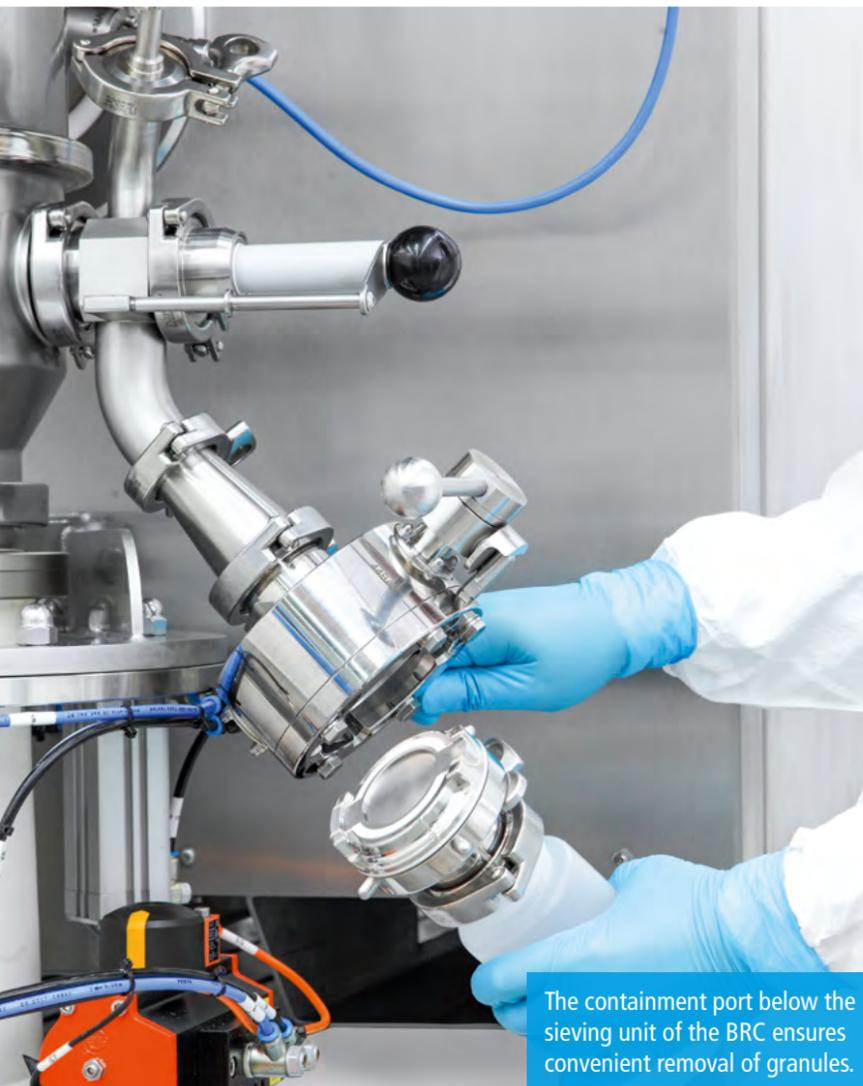
The containment port below the sieving unit of the BRC ensures convenient removal of granules.
